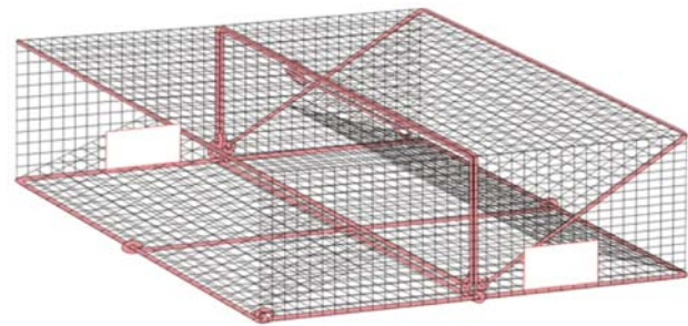
Fig. 5 Escape vents (35 × 45 mm) were located at both sides of the bottom at the side panel for the field fishing trials
